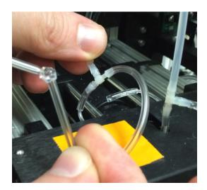
c) Now insert the syringe with tubing adaptors (should also be located in the small bin on top of the laser box) into the tube that was originally connected to the Timetian
