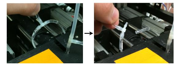
b) Connect the piece Tygon tubing that has been knotted off (should be located in small bin on top of the laser box) to the exposed part of the T-junction.
