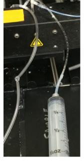
Once it is fully setup and tubes are securely connected, open the sheath valve in the Manual Control box. This will start flow both into the flow cell and into the syringe. Allow sheath flow for ~10 seconds. During that time, gently pull on the syringe, then release, and keep doing that to help remove the clog. When the syringe is full, close the sheath valve in the Manual Control box.
