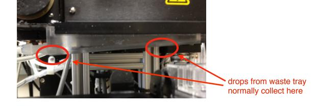
3) Make sure the sponge guard is always on. If it is off, and you put it on, be sure to slide it into position without disturbing the tubing too much. Too much disturbance can move the flow cell.
