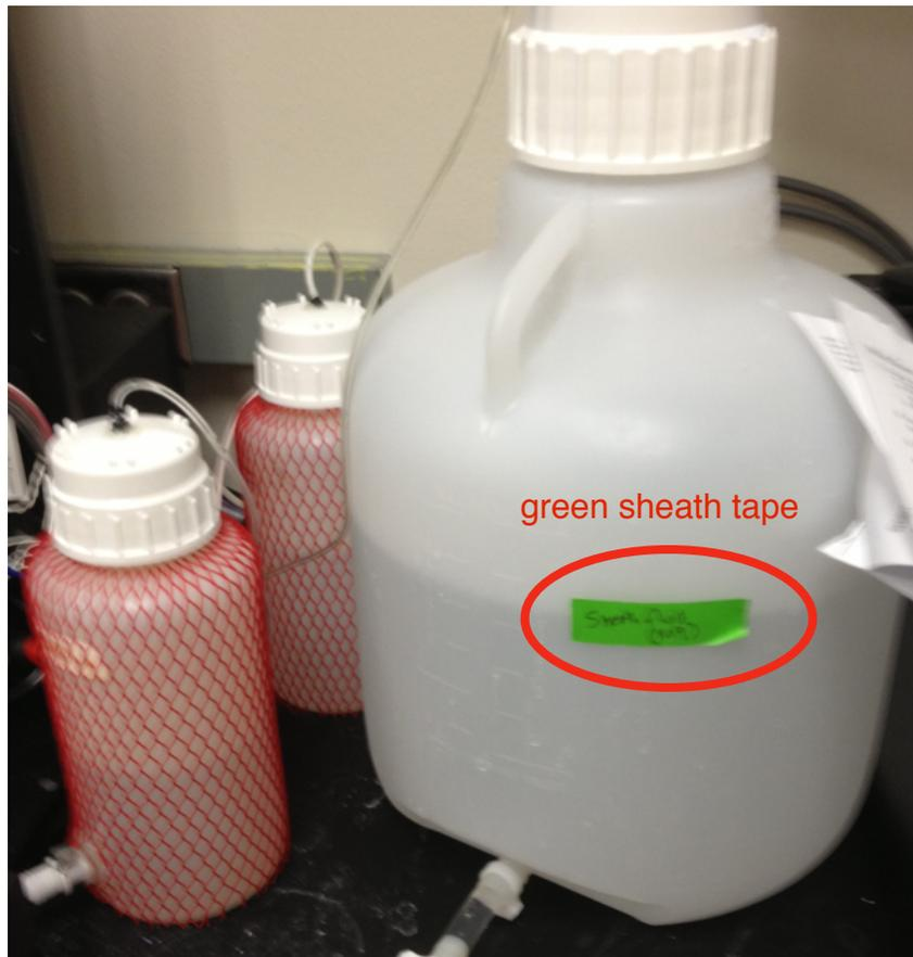
6) Make sure the clean and reflex bottles (red mesh bottles) are over one-third filled. If they are low on liquid, when the current plate finishes, uncheck “Sheath” in the Manual Control box. Unscrew the lids and add autoclaved water to the bottles. Do not fill higher than the fill line. Put the tops back on, re-check the “Sheath” in Pressure Status box. Wait for the sheath pressure to fully re-pressurize before running the next plate.
